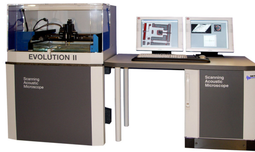
Fig. 1: SAM EVOLUTION II: Designed to operate in the frequency range from 3 MHz up to 400 MHz. It combines a high-speed high-resolution linear scanning system, a new developed high frequency electronic unit and a user friendly graphical working interface. A set of transducers is available for different types of applications.
